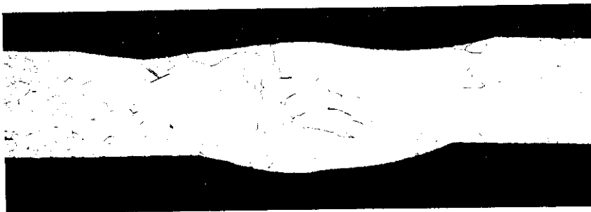
Steel A, 2mm thick, TIG 6 000 J/cm
