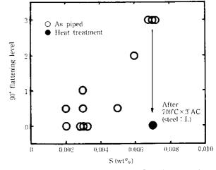
Fig. 8 Effect of S contents on 90° flattening properties
